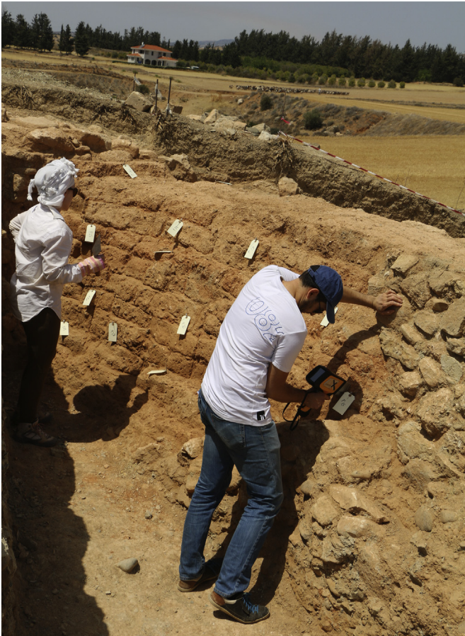
Fig. 8. pXRF performed on the NE curved section of the mudbricks (PULP 2016).
