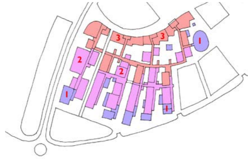
Testing the Site for the Faculty of Engineering, Building Heights
